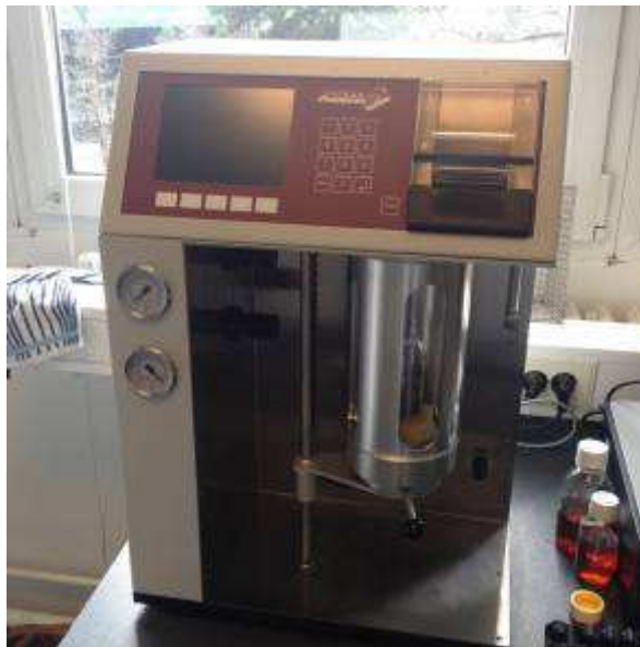
Figure 7: Equipment for testing hydraulic oil cleanliness
